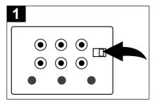
When connected to an external TV, slide this switch to the CAMERA position to see the image from the camera on the external TV. During playback of a CD+G disc, slide to the CDG position to see the song's lyrics on the external TV.
